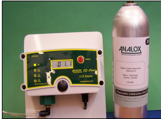
Connecting of the gas cylinder
